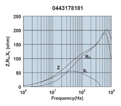
Impedance, reactance, and resistance vs. frequency.
