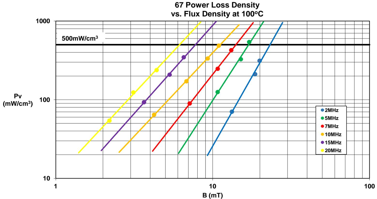
Measured on a 22.1mm/13.7mm/6.35mm toroid at 100° C.
