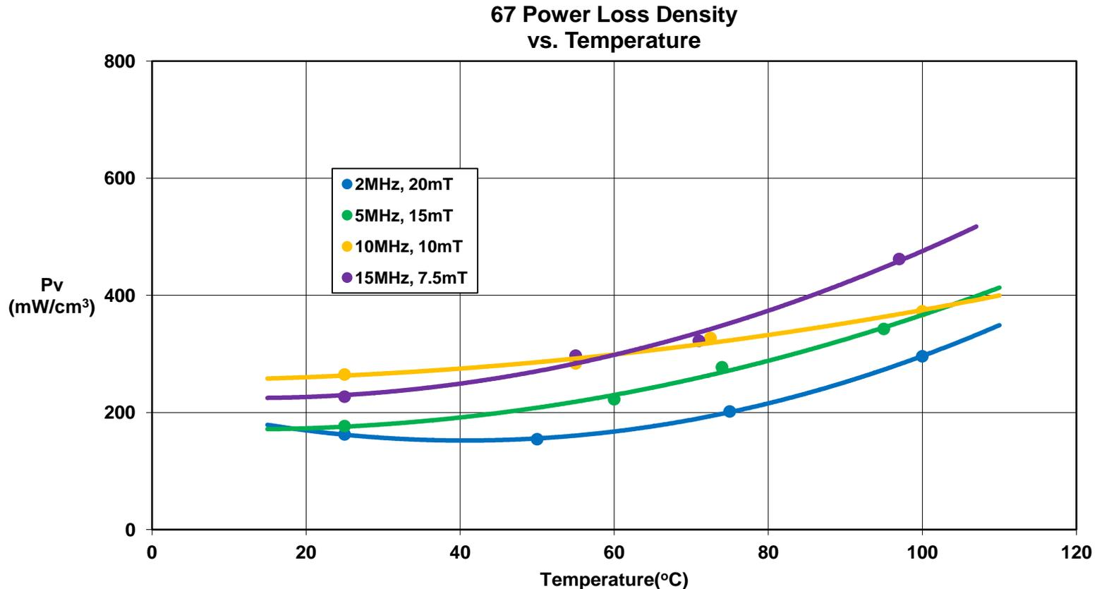
Measured on a 22.1mm/13.7mm/6.35mm toroid .
