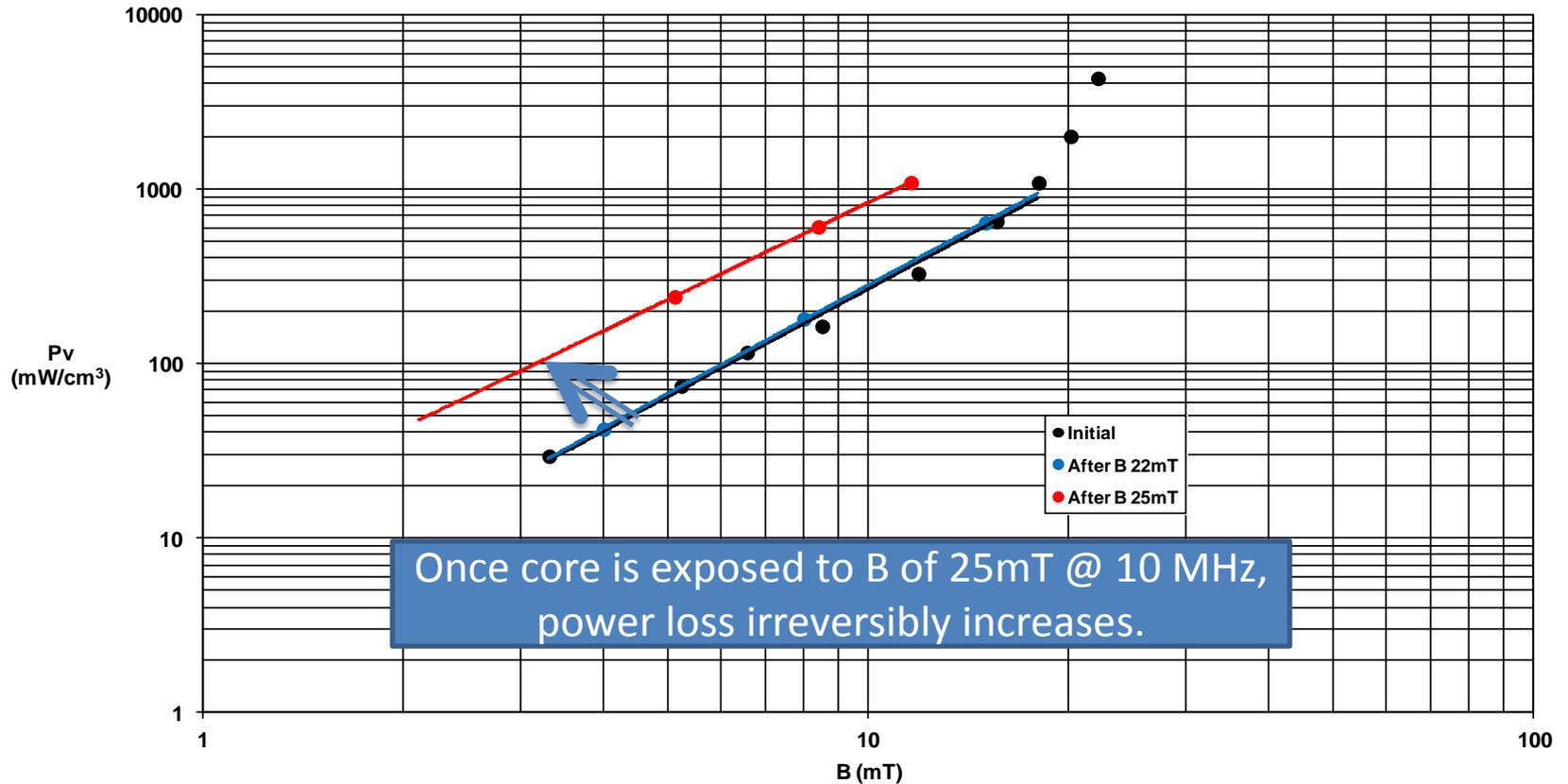
Once core is exposed to B of 25mT @ 10 MHz,
