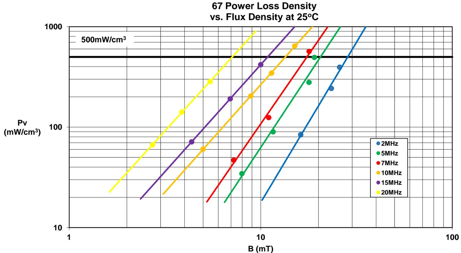
Measured on a 22.1mm/13.7mm/6.35mm toroid at 25°C.
