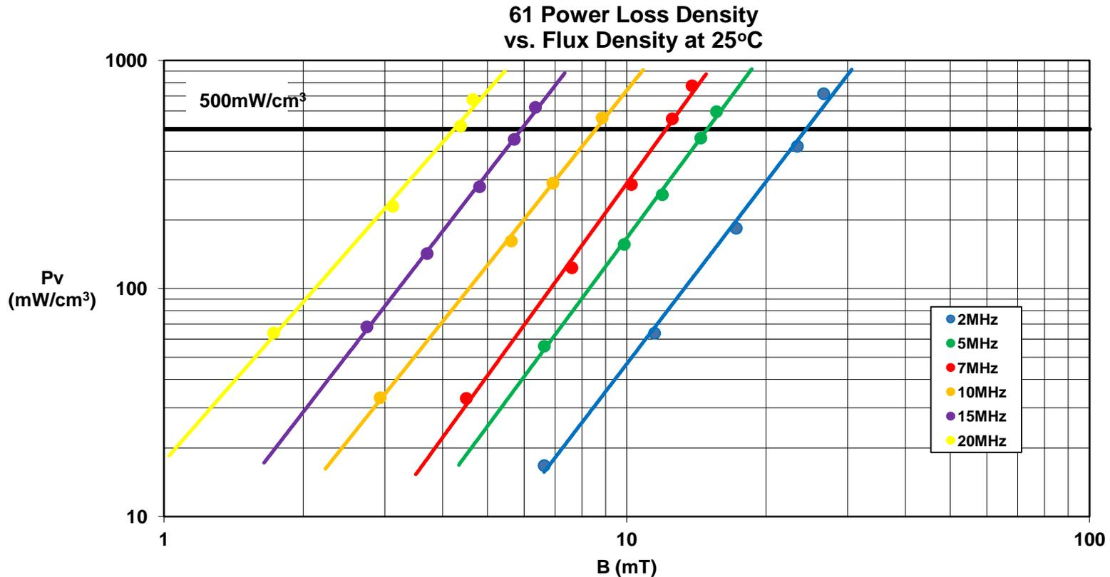
Measured on a 18.8mm/10.2mm/6.3mm toroid at 25 C.
