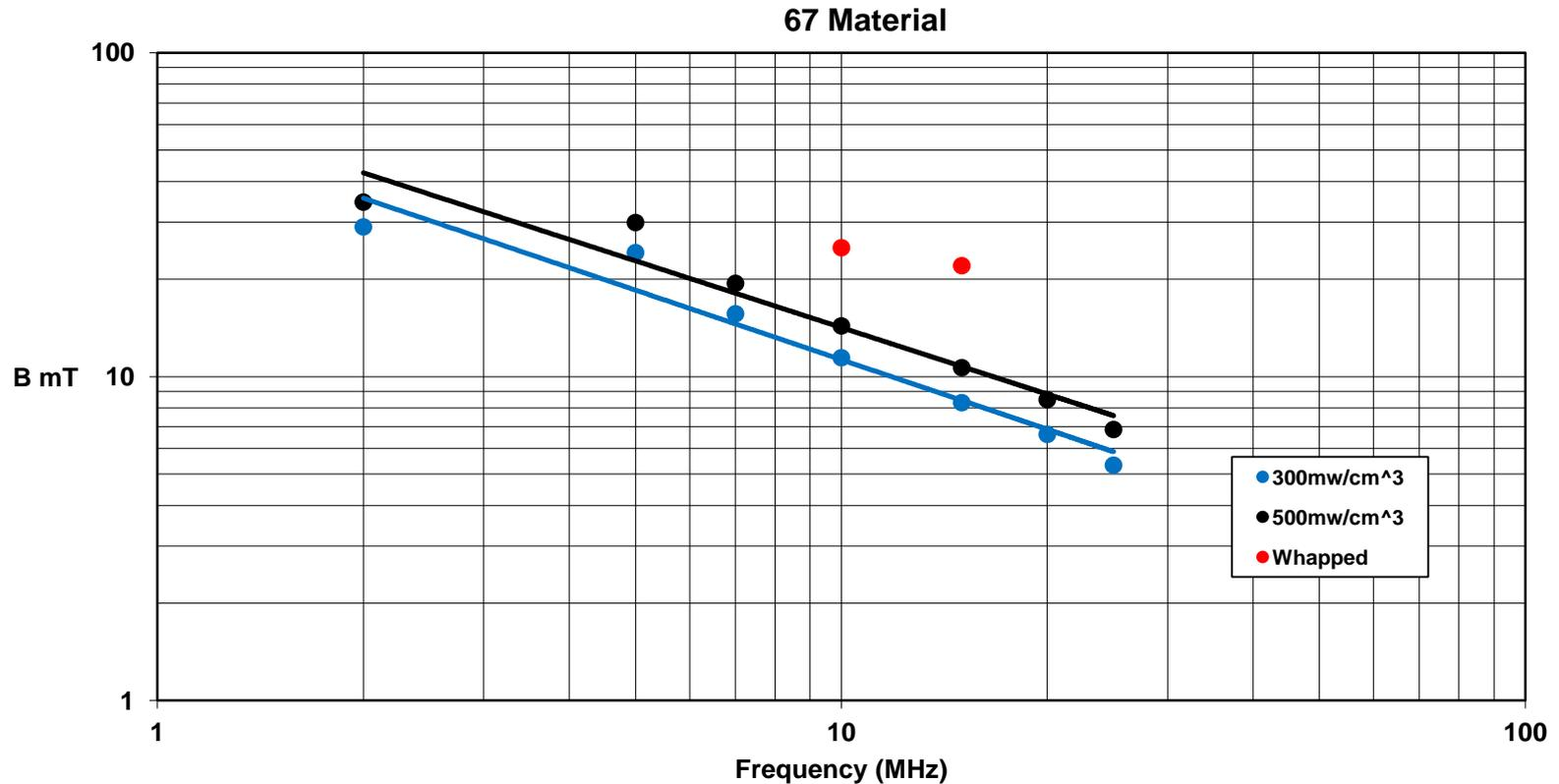
Measured on a 12.7mm/7.9mm/6.35mm toroid at 25° C.
