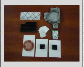
OC-800 is a thermally conductive phase change material having a softening temperature of 50-65°C. The liquid phase of the material can fill interface irregularities with much higher efficiency than traditional gap filler. On the other hand, it is a solid at room temperature and can be handled easily during installation.
