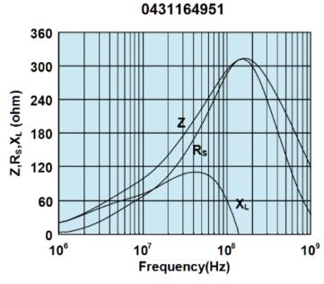
Impedance, reactance, and resistance vs. frequency.
